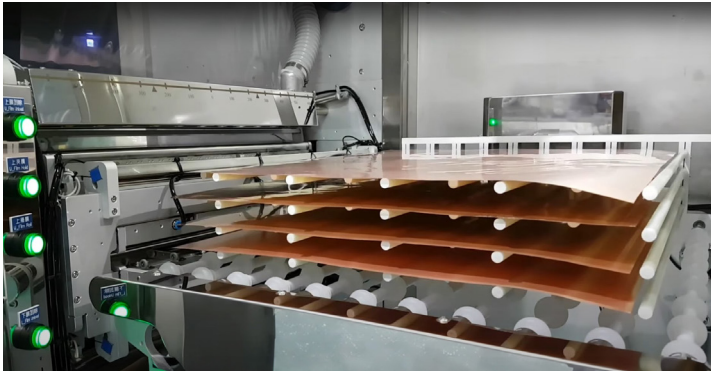
Exit Buffer for 4 Panels: gets activated if mylar is not removed.
